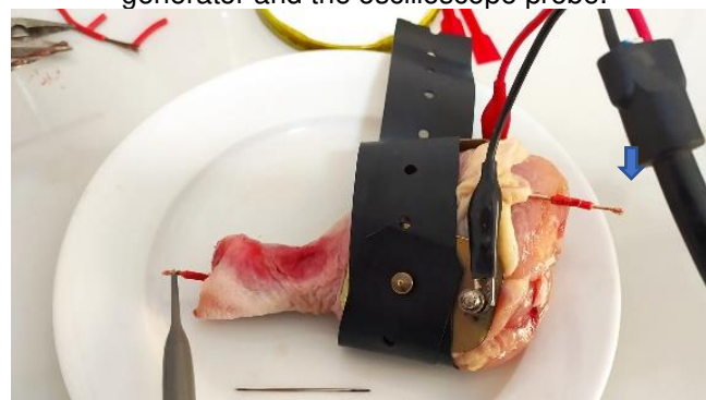
Figure 1. The anatomical structure of a bird connected to the EOI and connected to the incident wave generator and the oscilloscope probe.
